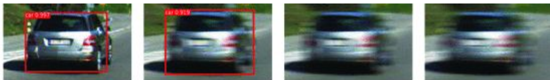
(a) Car detected without any motion blur (confidence score 0.997)
