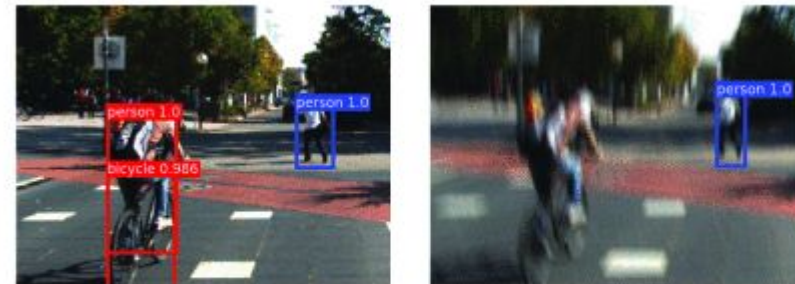
(b) The person and bicycle in the clear image (left) is hidden after blurring (right).
