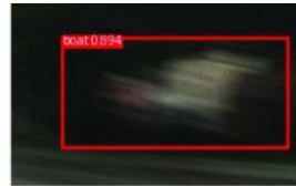
(c) Boat detected (0.894) after linear motion blur (heavy, inclined)
