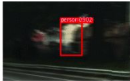
(b) Person detected (0.902) after linear motion blur (slight, horizontal)
