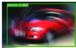
(d) Car is misclassified as person (0.969) after rotational motion blur (heavy, anticlockwise)
