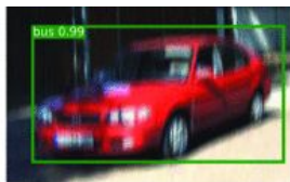
(b) Car is misclassified as bus (0.99) after linear motion blur (slight, vertical)
