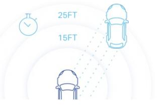
The sensor uses the time it took for each pulse to return to the sensor to calculate the distance it traveled
