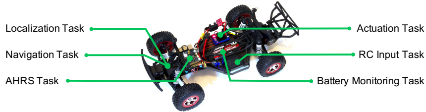
Figure 1.1: A rover system that exemplifies a typical real-time system. This system consists of six real-time periodic tasks that support an autopilot feature.
